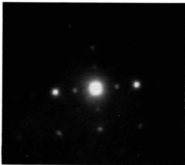
Fig. 1. Pattern from AuCu film (500 Å in thickness) as evaporated showing tetragonal AuCu I.
