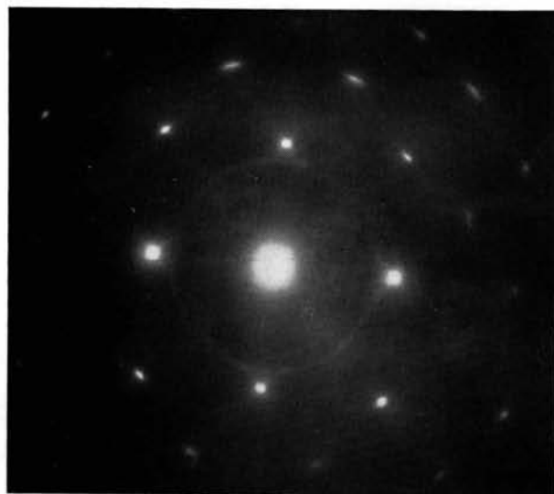
Fig. 4. Pattern from same single crystal film at 450 °C. showing intensities in reciprocal space corresponding to f.c.c. lattice.
